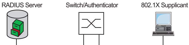
Figure 25: Radius server connection
